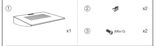
1 Place the sliding nuts2 approximately 370 mm apart. Push them into the toolbar T-slot, then turn to make the spring face away from you.
