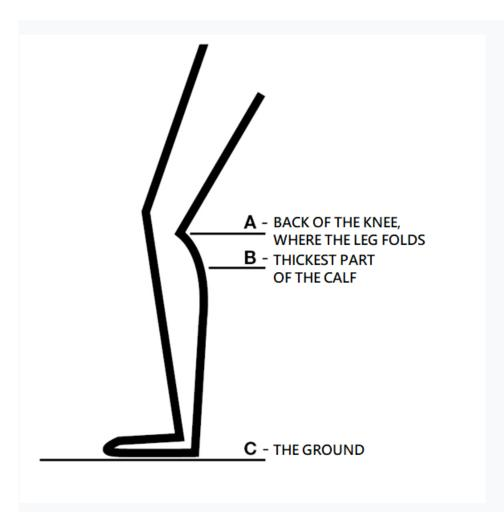
Measure with a tape measure on the leg between points A and C and compare with the table above which stilt should be used. Length must not be exceeded.
