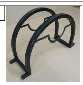
Take the 15cm smallest square tubes and connect the two arches together.
