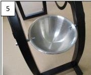
Fix on a small bowl. You may find it easier to position the bowl, then thread the screw through the hole not forgetting the spacer). Attach a nyloc nut but do not tighten yet.
