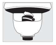
To focus the projected effect, twist the slide on the lens forward and backwards until your desired focus is achieved.
