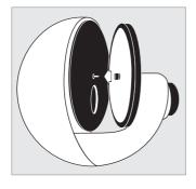
To attach plastic bossed push-on effect wheels, simply push the wheels onto the shaft of the wheel rotator as per the image left.
