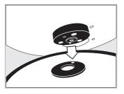
Position the magnetic wheel onto the magnetic adaptor on the projector.
