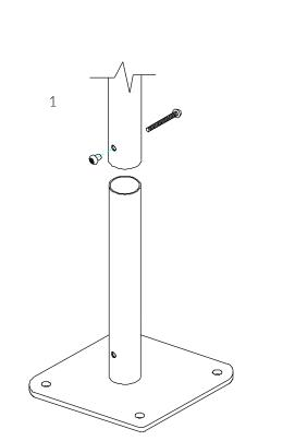
Locate the Surface fix Plate into the leg of the instrument. Fix instrument to Surface fix plate using M10 bolt and Barrel Nut and use **thread locking solution** to prevent fixings working loose.
